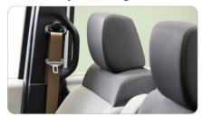
Neck impact mitigation seats are installed in the driver and passenger seats, which reduce the strain on the neck in case hit from behind at a low-speed
